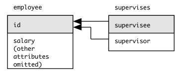
(The names of the attributes of the supervises table denote <u>roles</u>, and are similar in meaning to the use of roles when labelling an association in a UML class diagram. Of course, supervisor and supervisee are actually employee ids)
